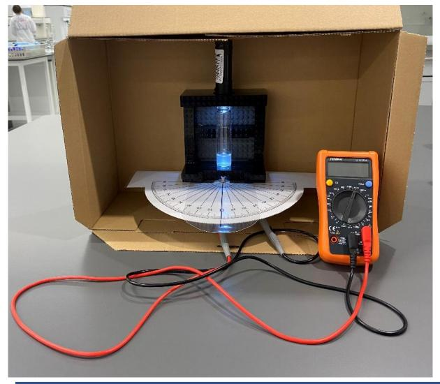
Tip: Construction of Lego® Polarimeter
