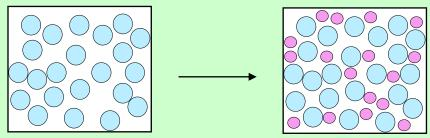
The **more solid** that is added to water, the **denser** the solution is that is made, as more of the space between the water molecules is being filled.
