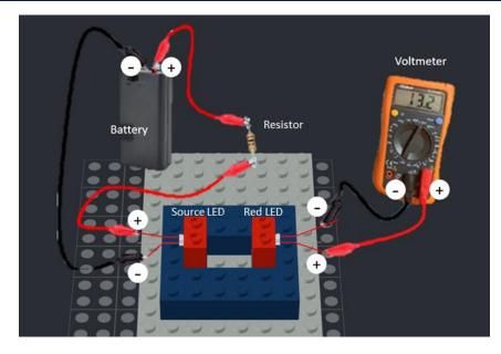
Turn the multimeter to the 2000m (2000 mV) direct voltage setting. If the source LED is lit up, this should produce a non-zero reading of roughly 600 - 1000 mV. You should also be able to observe that the voltage reading drops if something, such as a finger, is inserted to obstruct the light path between the two LEDs.
