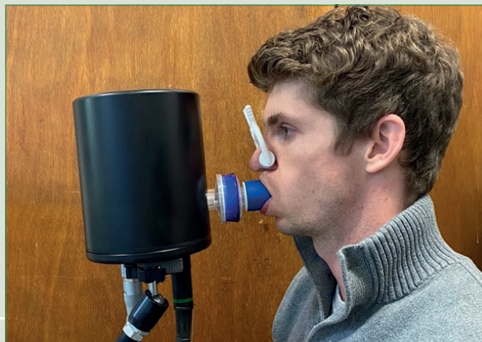
Figure 1: The laser gas analyser in use, demonstrated by Dr Nick Smith, one of the chemists who developed it. The device is housed in the black box, which is breathed into by the subject using a mouthpiece and noseclip to ensure that all inhaled and exhaled gases enter the device.
